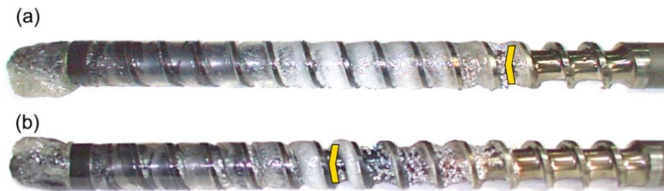
Figure 13. An effect of the plastication stroke on the polymer flow in the injection molding process at the screw speed N = 300 rpm, and the back pressure P_{\text{back}} = 0 MPa: (a) h_{\text{plast}} = 1 D , (b) h_{\text{plast}} = 3 D .
