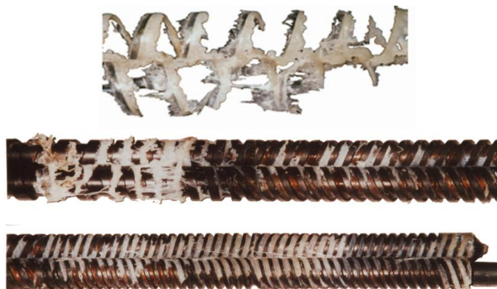
Figure 5. Melting mechanism observed in counter-rotating twin screw extrusion [74].
