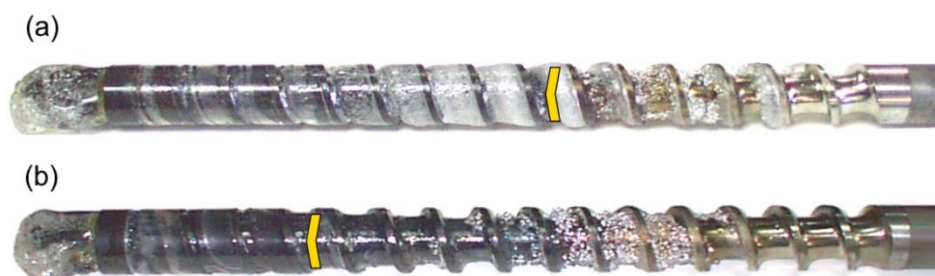
Figure 11. An effect of the plastification stroke on the polymer flow in the injection molding process at the screw speed N = 100 \text{ rpm} , and the back pressure P_{\text{back}} = 0 \text{ MPa} : (a) h_{\text{plast}} = 1 D , (b) h_{\text{plast}} = 3 D .
