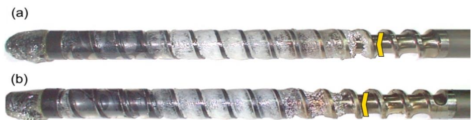
Figure 15. An effect of the plastication stroke on the polymer flow in the injection molding process at the screw speed N = 300 rpm, and the back pressure P_{\text{back}} = 3 MPa: (a) h_{\text{plast}} = 1 D , (b) h_{\text{plast}} = 3 D .
