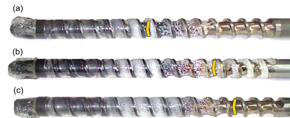
Figure 19. An effect of the back pressure on the polymer flow in the injection molding process at the screw speed N = 300 rpm, and the plasticating stroke h_{\text{plast}} = 3 D : (a) P_{\text{back}} = 0 MPa, (b) P_{\text{back}} = 2 MPa, (c) P_{\text{back}} = 3 MPa.
