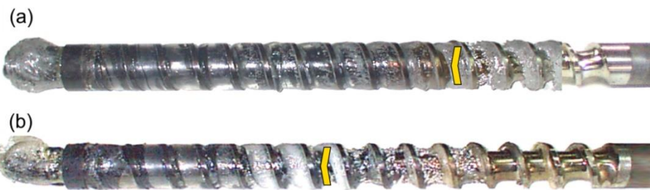
Figure 12. An effect of the plastication stroke on the polymer flow in the injection molding process at the screw speed N = 100 rpm, and the back pressure P_{\text{back}} = 2 MPa: (a) h_{\text{plast}} = 1 D , (b) h_{\text{plast}} = 3 D .
