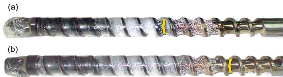
Figure 10. An effect of the screw speed on the polymer flow in the injection molding process at the plastification stroke h_{\text{plast}} = 3 D , and the back pressure P_{\text{back}} = 3 \text{ MPa} : (a) N = 100 \text{ rpm} , (b) N = 300 \text{ rpm} .
