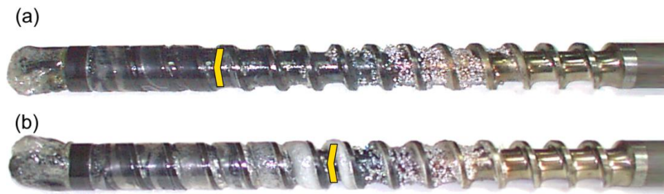
Figure 8. An effect of the screw speed on the polymer flow in the injection molding process at the plastification stroke h_{\text{plast}} = 3 D , and the back pressure P_{\text{back}} = 0 \text{ MPa} : (a) N = 100 \text{ rpm} , (b) N = 300 \text{ rpm} .
