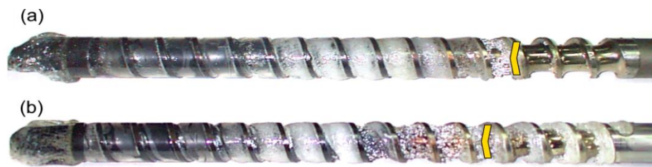
Figure 14. An effect of the plastication stroke on the polymer flow in the injection molding process at the screw speed N = 300 rpm, and the back pressure P_{\text{back}} = 2 MPa: (a) h_{\text{plast}} = 1 D , (b) h_{\text{plast}} = 3 D .
