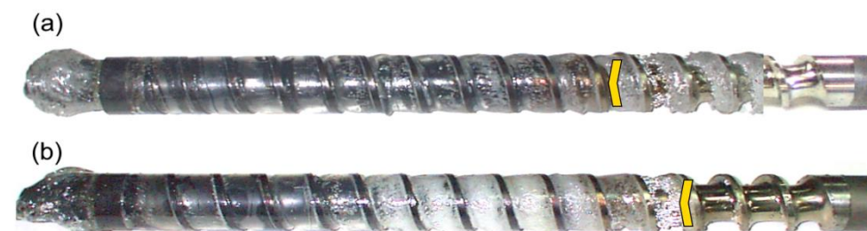
Figure 7. An effect of the screw speed on the polymer flow in the injection molding process at the plastication stroke h_{\text{plast}} = 1 D , and the back pressure P_{\text{back}} = 2 \text{ MPa} : (a) N = 100 \text{ rpm} , (b) N = 300 \text{ rpm} .
