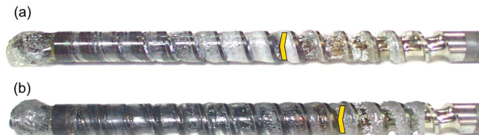
Figure 16. An effect of the back pressure on the polymer flow in the injection molding process at the screw speed N = 100 rpm, and the plasticating stroke h_{\text{plast}} = 1 D : (a) P_{\text{back}} = 0 MPa, (b) P_{\text{back}} = 2 MPa.
