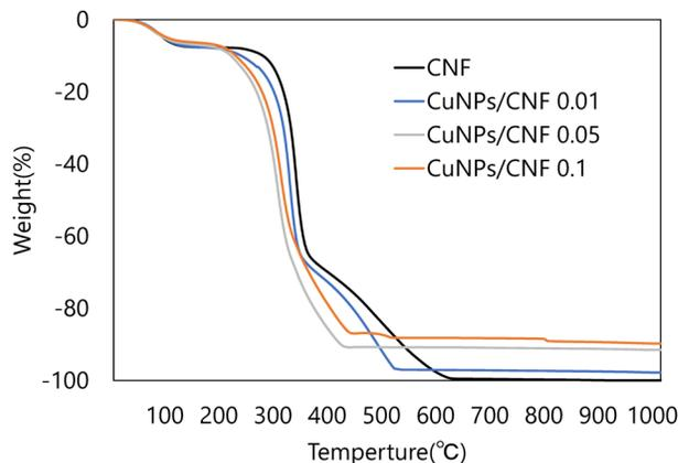
Fig. 3. Thermogravimetric analysis curve of CuNPs/CNF composites.
