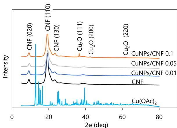
Fig. 2. XRD profiles of CuNPs/CNF composites.
