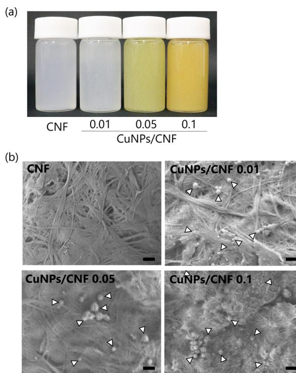
**Fig. 1.** CuNPs/CNF composites. (a) Color of CuNPs/CNF composites. CNF was mixed with different concentrations of copper acetate at 0.01, 0.05, and 0.1 M. (b) Field-emission scanning electron microscopy micrographs of CNF and CuNPs/CNF composites. Arrowheads indicate copper particles. Bars indicate 500 nm.
