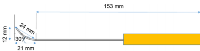
Figure 3. MicroSutureLasso Minor Bend (Arthrex) with a 30° curved tip. The lengths of the tip and shaft were 24 and 153 mm, respectively.
