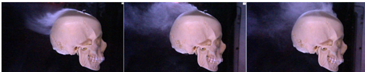
FIG. 10. Frame sequence from high-speed imaging of blast-wave exposure of ‘free-flight’ human-skull replica showing flow patterns; negligible motion was imparted for a blast of 125 kPa and 6 ms duration. (reprinted with permission from Ritzel and colleagues 44 ).
