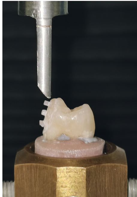
FIGURE 3: Microshear bond strength test using universal testing machine.
