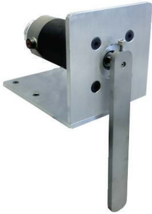
FIGURE 9: Experimental one-degree-of-freedom arm (pendulum) subject to gravitational force.
