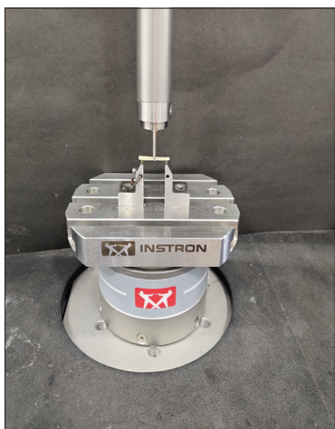
Figure 1: The image depicts the determination of maximum force with INSTRON E3000 (Electroplus) universal testing machine
