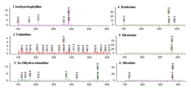
Figure 2. Positive fragments of alkaloids present in Uncaria rhynchophylla extract and characterization of six representative components assessed by HPLC-MS.
