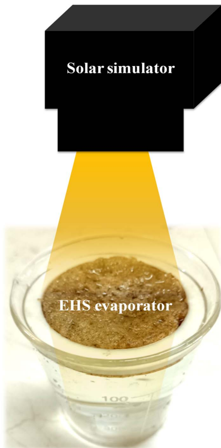
Fig. 3 Solar steam generation experimental setup.
