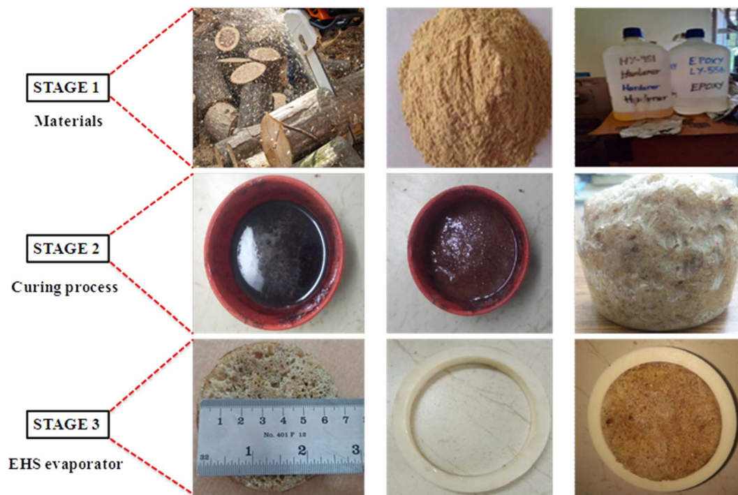
Fig. 2 Fabrication of the circular type epoxy/hardener/sawdust composite.
