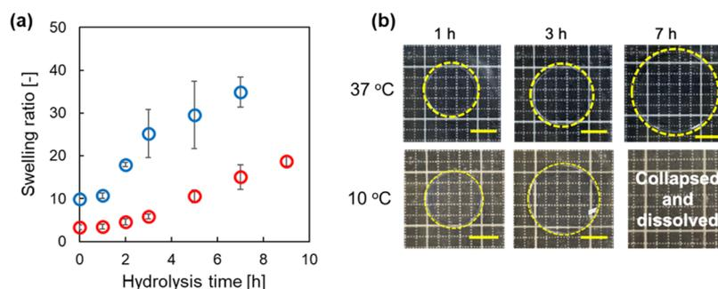
**Figure 2.** Characterization of hydrogels during alkaline hydrolysis. Hydrogels prepared with the composition of (MDO + HEA)/PEGMA = 100:1 (mol/mol) and MDO/HEA = 6:4 (mol/mol). (a) Hydrolysis time-dependent changes in swelling ratios of the hydrogels at 37 and 10 °C. Data are expressed as the mean  $\pm$  SD ( $n = 3$ ). Red plot: 37 °C and blue plot: 10 °C. (b) Optical images of the hydrogel during hydrolysis at 10 and 37 °C.
