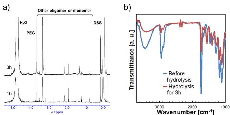
**Figure 3.** Characterization of the hydrogel surface and degradation supernatant during alkaline hydrolysis. Hydrogels were prepared with the composition of (MDO + HEA)/PEGMA = 100:1 (mol/mol) and MDO/HEA = 6:4 (mol/mol). (a) <sup>1</sup>H NMR spectra of supernatants during hydrolysis of hydrogels for 1 and 3 h. (b) ATR-FTIR spectra of dried hydrogels before and after hydrolysis for 3 h.
