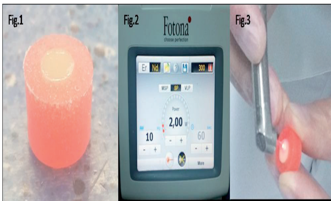
Figure 1, 2 and 3. From left to right: An example of porcelain disc, the laser system used in the study and laser treatment of porcelain surface.
