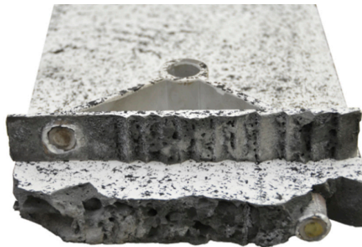
Figure 29. Failure mode of implant type 5—failure of the weld seam.
