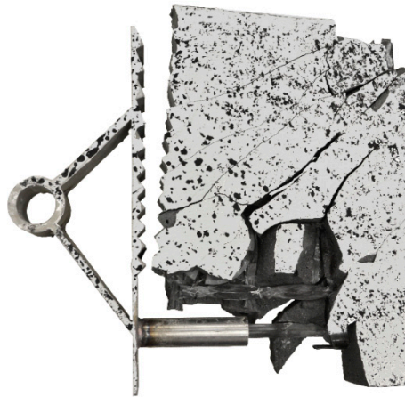
Figure 26. Failure mode of implant type 2—pulling out of the carbon rod from the anchorage.
