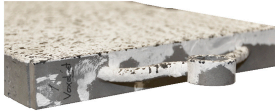
Figure 31. Failure mode of implant type 7—deformed compression strut of the implant.
