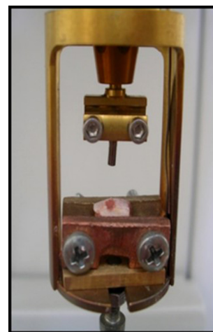
Fig. 2 A. Mechanical characterization of the ex-vivo sample using the Dynamic Mechanical Analyzer (DMA 7-e): sample mounted: showing the bone attached to the lower member and the pin attached to the upper member of the assembly, titanium rod pulled-out of place,
