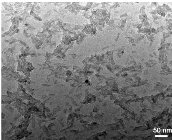
**Figure 1** Transmission electron microscope image of nano-hydroxyapatite.
