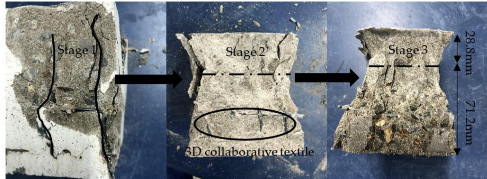
Figure 5. Failure mode of 3D-TRSSC ultimate strength.
