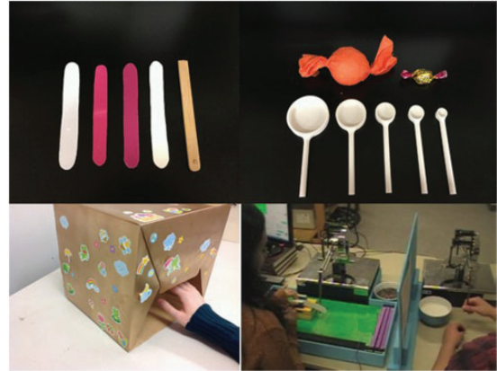
Figure 1. Materials Function Judgment Task: Sticks (upper left) and spoons (upper right); box for No Tech condition (lower left); teleoperated robot for Tech condition (lower right). The participant is moving the end effector of the user-side robot on the right side of the barrier which moves the end effector of the environment-side robot on the left side of the barrier. The researcher on the left is stabilizing a stick in place while the user explores it. A bowl of sugar is visible to the user on the right side of the panel.
