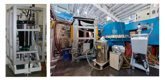
**Figure 1.** Neutron protein crystallography instrumentation. (**Left**) photograph of the LADI-III Quasi-Laue diffractometer, located at the Institut Laue-Langevin, Grenoble FR [19]; (**Right**) photograph of the BIODIFF monochromatic diffractometer, located at Heinz Maier-Leibnitz Zentrum, Munich DE. Re-used with permission from the photographer, Bernhard Ludewig.
