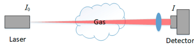
Figure 1. Laser absorption spectroscopy concept.
