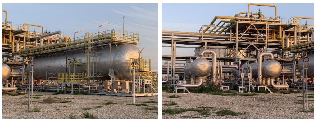
Figure 1. The side view and front view of the practical oil–water separator studied in this paper.
