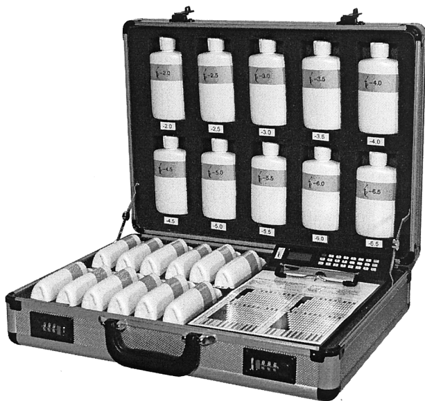
Fig. 2. The Smell Threshold Test™, a commercially available test for assessing odor detection thresholds. Concentrations of phenyl ethyl alcohol, ranging from 10^{-2} to 10^{-10} log vol/vol in half-log concentration steps, are provided, along with blanks for forced-choice testing. (Photograph courtesy of Sensonics, Inc., Haddon Heights, NJ. Copyright 2000, Sensonics, Inc.)
