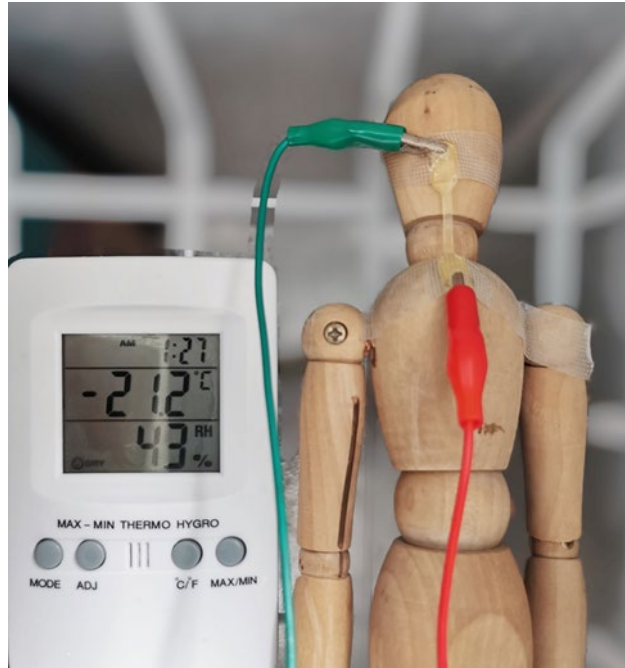
Supplementary Figure 21. The digital photograph of sensing ability test at subzero temperatures.
