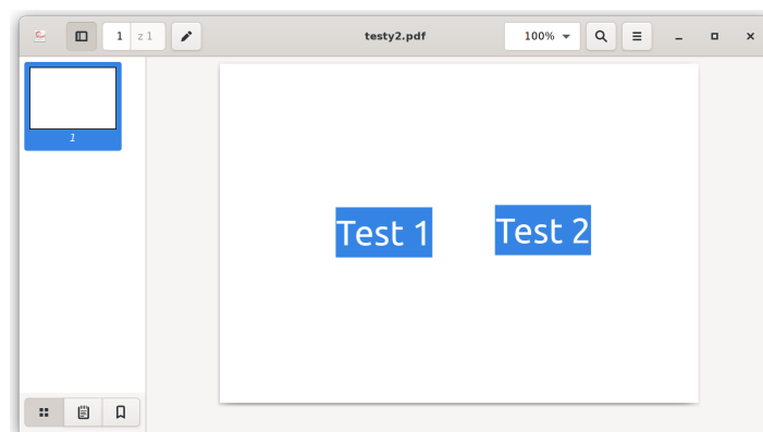
Figure 4. Example of different technique—hiding text by changing color or covering it with a rectangle.
