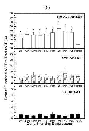
**Figure 8.** Effect of viral gene silencing suppressors on extracellular total rAAT production (**A**), extracellular functional rAAT production (**B**), and ratio of functional rAAT to total rAAT (**C**) in transgenic plant cell cultures (CMViva, XVE or 35S). Error bars represent one standard deviation of measurements obtained from triplicate sample assays of duplicate experiments. Asterisks on the graphs indicate a statistically significant difference from the control ( $p \le 0.05$ ).
