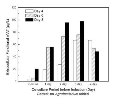
Figure 7. Investigations of the effect of induction timing after starting co-cultivation process on rAAT production. The inducer was added into the co-culture process of *Agrobacterium* carrying viral gene silencing suppressor P19 with transgenic CMViva on days 1, 2, 3 and 4 after agroinfiltration in a 6-well microplate at 20  $^{\circ}$ C. The biomass ratio of *Agrobacterium* to plant cell was 25  $\mu$ g-DCW/g-DCW. Samples were taken on days 4, 6 and 8 post-induction.
