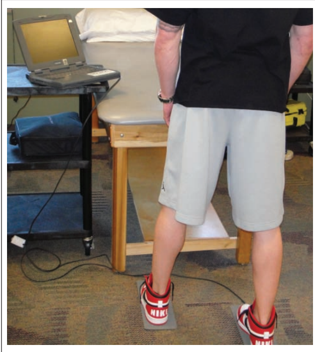
Figure 1. Initial weightbearing exercises such as a weight shift can be performed on a force platform that can measure the amount of weight distribution between each extremity.
