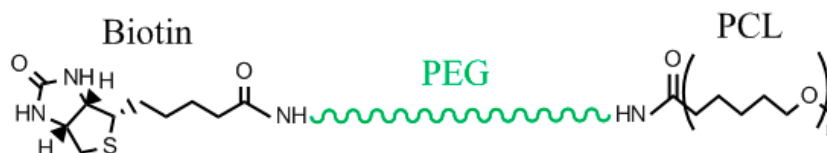
Figure 2. Chemical connectivity of PCL-PEG-Biotin nanoparticle design.
