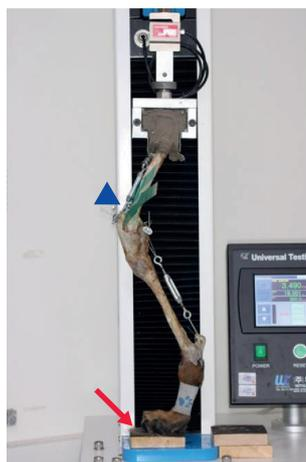
**Fig. 2.** The prepared specimens were mounted on Universal Testing Machine. The Sandpaper was attached on contact area of palmar pad to prevent slipping (red arrow). There is pressure distribution sensor in patellofemoral joint (blue arrowhead).
