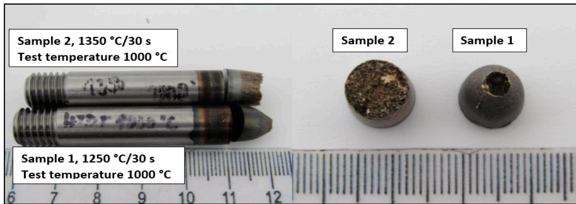
Figure 3. Macro-view of samples after hot ductility test.
