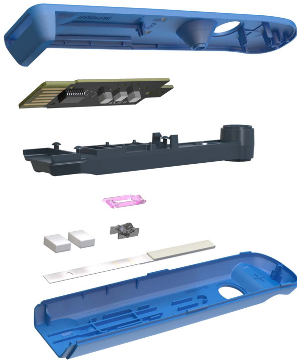
Figure 1 QIAreach QFT digital detection cartridge (eStick). Exploded QIAreach QFT eStick. Casing (blue) contains lateral flow assay strip with optoelectronic technology and a micro-processor that converts a fluorescent signal into a qualitative readout for the detection of interferon-gamma in the plasma sample that has been stimulated by peptide antigens that are associated with M. tuberculosis .
