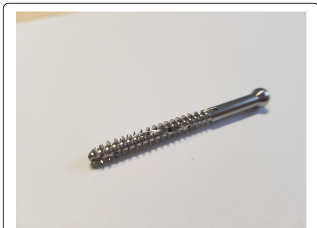
Fig. 2 Illustration of the new, partially threaded, fenestrated, cancellous, condylar screw (diameter 5 mm) suitable for the NCB ® -DF system. The screw provides two longitudinal furrows and ten perforation holes, for an optimal cement extrusion along the shaft of the screw
