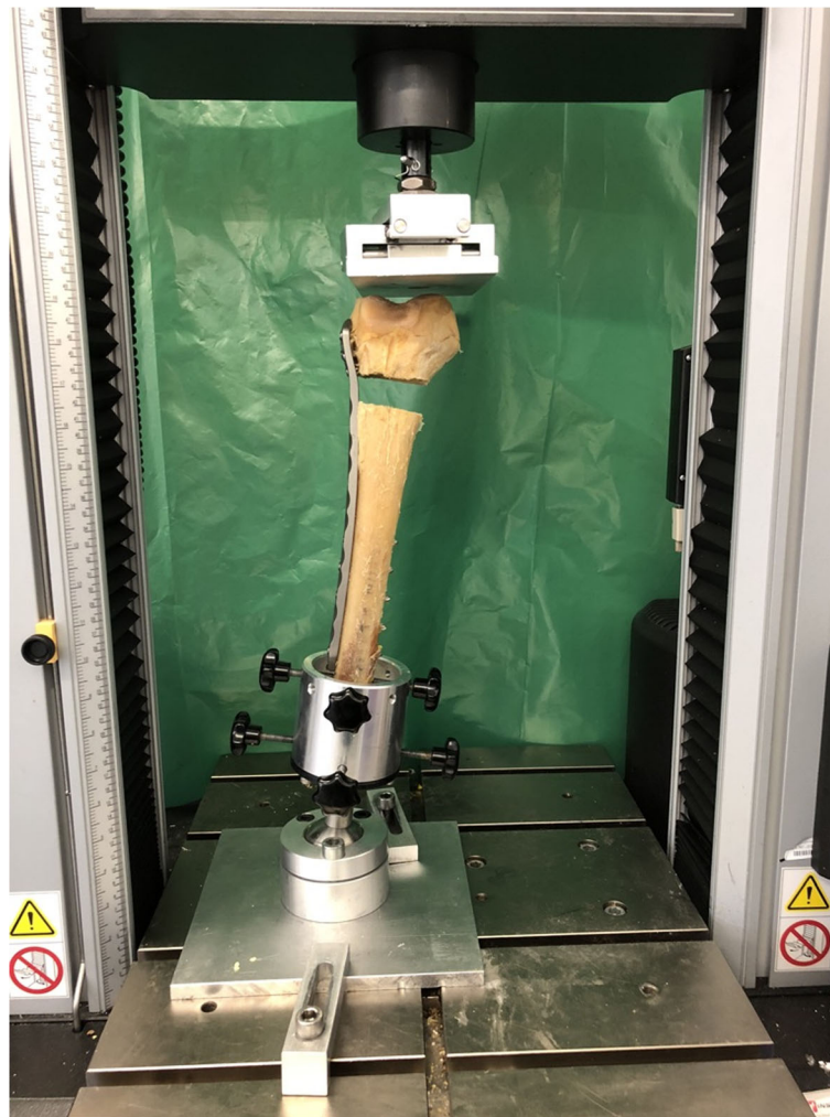
Fig. 5 Test setup demonstrating force application with a metal plate, movable in two directions. The femoral shaft is statically fixed in an anatomical 5–7° valgus position
