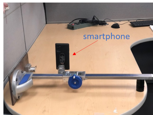
Figure 12. Linear rail set up for inducing translational camera motion.
