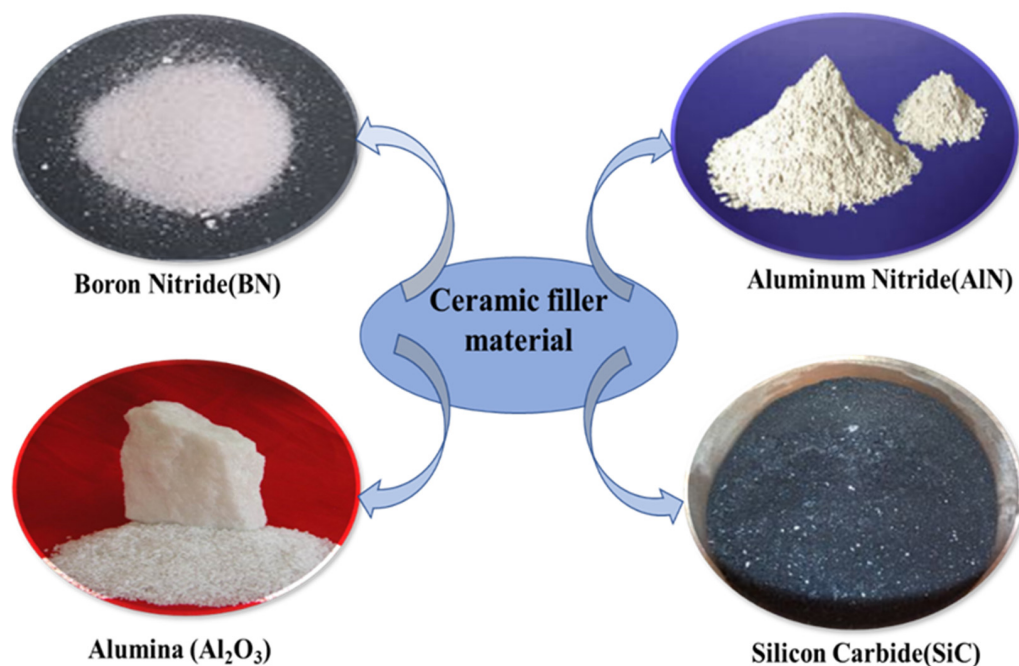
Figure 5. Commonly used thermally conductive ceramics filler.
