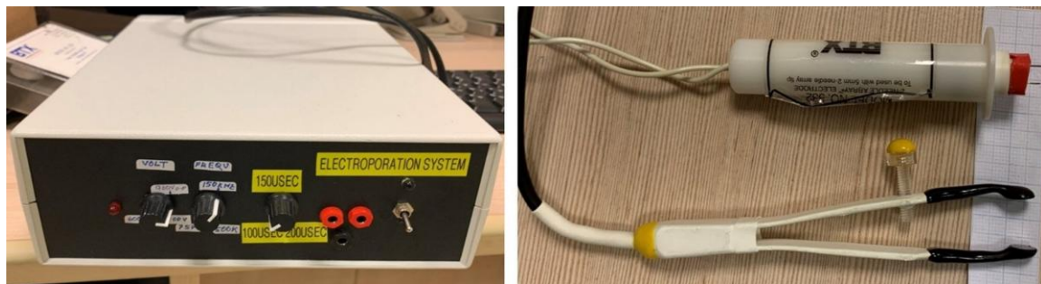
Figure 1 Equipment description and configuration; (left) a custom-made generator based on an H bridge circuit consisting of four N and P channels MOSFET. The generator enables a maximal output voltage of 1100 V, at a frequency range of 75–150 kHz with burst duration between 100 and 200 \mu s. (Right) Two needle electrodes (top) with 3 mm in length and with 5 mm distance between them and (bottom) two-clamp electrodes (0.5 mm in diameter) with 0.5 cm inter-electrode distance.
