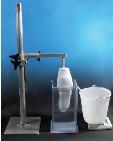
FIGURE 1: Water weighting of residual limb covered with one layer of Terry Cloth sock.
