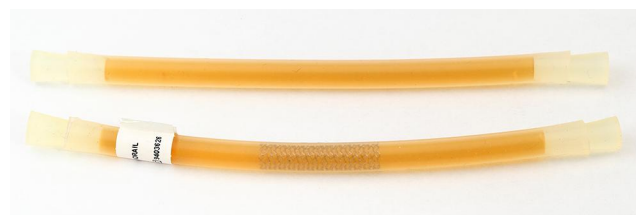
Figure 1 Image of a reference phantom (top) and a stented vessel phantom (bottom, Taxus Liberté 5/32), both filled with tracer dilution (1:100, Resovist, from Pharmaceuticals, Tokyo, Japan). The stented phantom has a slightly curved shape caused by the storage of the phantoms as wound tubes. For imaging, all phantoms were straightly aligned on a dedicated phantom holder.
