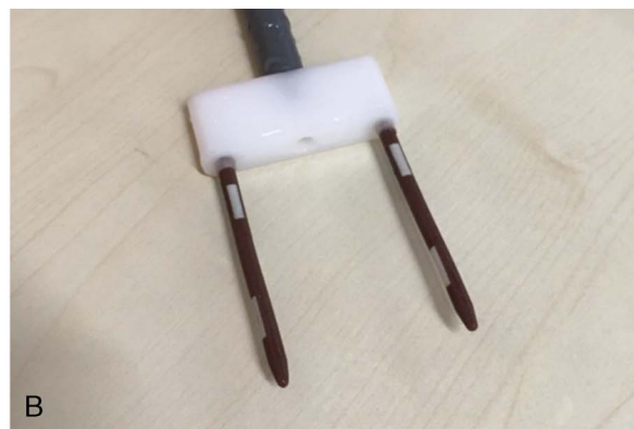
FIGURE 1. A, Cross-sectional drawing of the artificial vessel with 4 mm diameter containing 3 calcified lesions (QRM, Moehrendorf, Germany). The calcified lesions were manufactured to contain 800 mg/mL hydroxyapatite. B, Photograph of the carrier mounted vessels with the calcified lesions clearly visible. The mounting on the same carrier enabled simultaneous measurement in the cardiac motion phantom.
