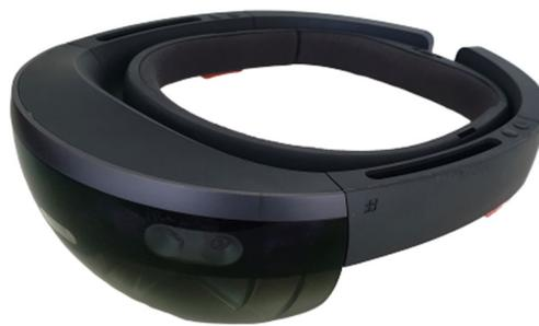
**Fig. 1** Augmented reality head-mounted display (HoloLens, Microsoft, Redmond, USA)
