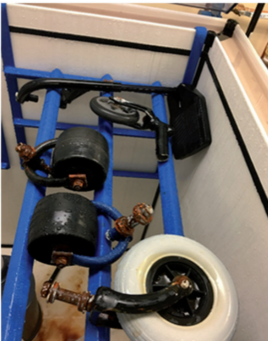
Figure 4. Salt fog test equipment for corrosion exposure. 21
