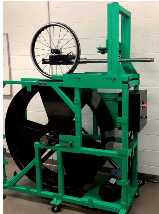
Figure 2. Drum based RR test equipment. 9
