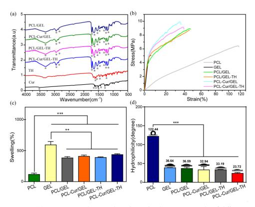
**Figure 2.** (a) FTIR spectra, the asterisks indicate the characteristic peaks of different samples. (b) Stress-strain curves. (c) Swelling abilities and (d) Water CAs (n = 3) of different nanofibrous membranes; \* p < 0.05; \*\* p < 0.01; \*\*\* p < 0.001.
