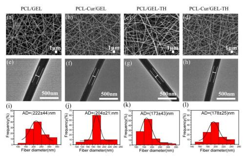
**Figure 1.** (**a**–**d**) SEM, (**e**–**h**) TEM images and (**i**–**l**) the corresponding diameter distribution of different coaxial nanofibers. The white dash line in (**e**–**h**) indicates the border between the PCL core and GEL shell.
