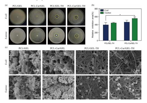
**Figure 4.** Antibacterial activity of different samples against *E. coli* and *S. aureus*. (a) Inhibition zone analysis. The yellow dotted circle in the figure is the inhibition zone. (b) Inhibition area of different samples (n = 3). (c) SEM images of *E. coli* and *S. aureus* on different membranes. \* p < 0.05.
