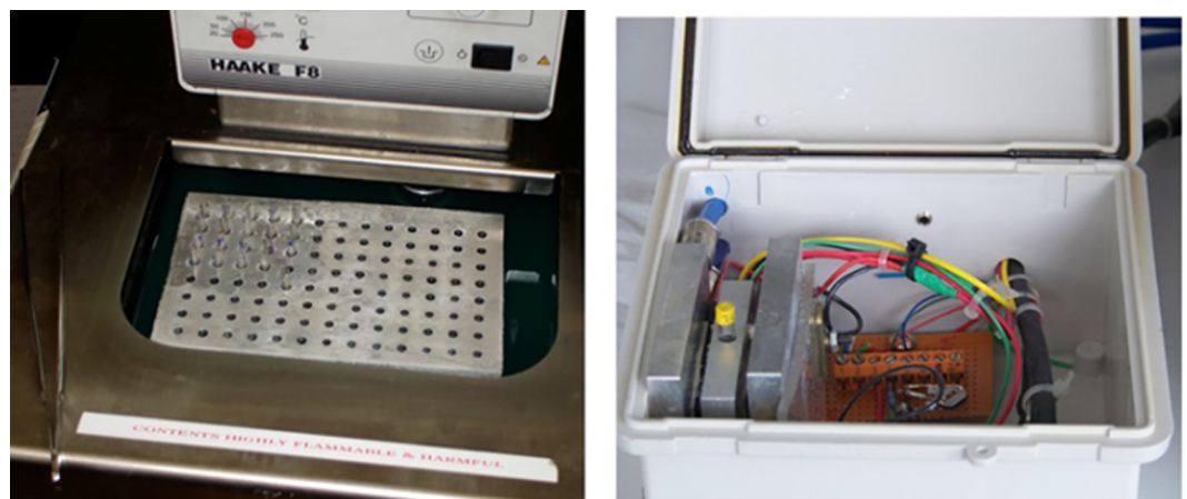
Fig 1. (Left) Metal rack holding the sample tubes, partly immersed in the ethanol bath of a refrigerated circulator. (Right) Sample chamber of the optical recrystallometer apparatus used for measuring RI activity.
