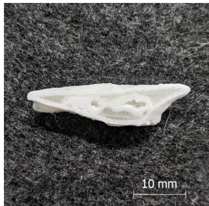
Figure 5. Structure of a printed performance implant (implant B, top view, cut at Z = 8 mm); white: TPU shell, transparent: PETG core.
