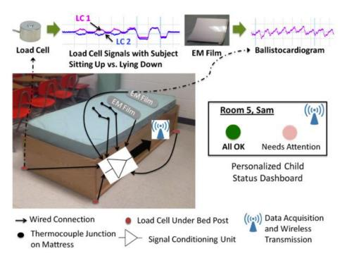
**Figure 8.** The bed sensor suite and the residential dashboard interface indicating the real-time status of the child on the bed. Sample data shows movements and ballistocardiogram (BCG) data (©2014 IEEE. Reprinted with permission [128]).
