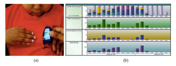
**Figure 7.** The Language ENvironment Analysis (LENA) device. (a) Custom-designed clothing with a pocket to insert the recorder; (b) Software interface of LENA showing the audio environment, child's vocalizations, conversational turns and adult words throughout the day. Images courtesy of Dr. M. Aldosari, Cleveland Clinic.
