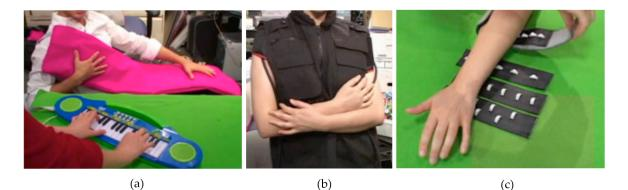
**Figure 5.** Various experimental haptic interfaces for therapy: (**a**) Touch Me simulates touch; (**b**) Squeeze Me simulates hugs; (**c**) Hurt Me induces controlled pain. (©2009 ACM. Reprinted with permission [80]).
