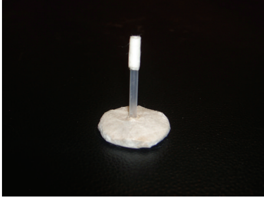
FIGURE 2: A small brass cylinder holds the acupuncture needle on the control side.
