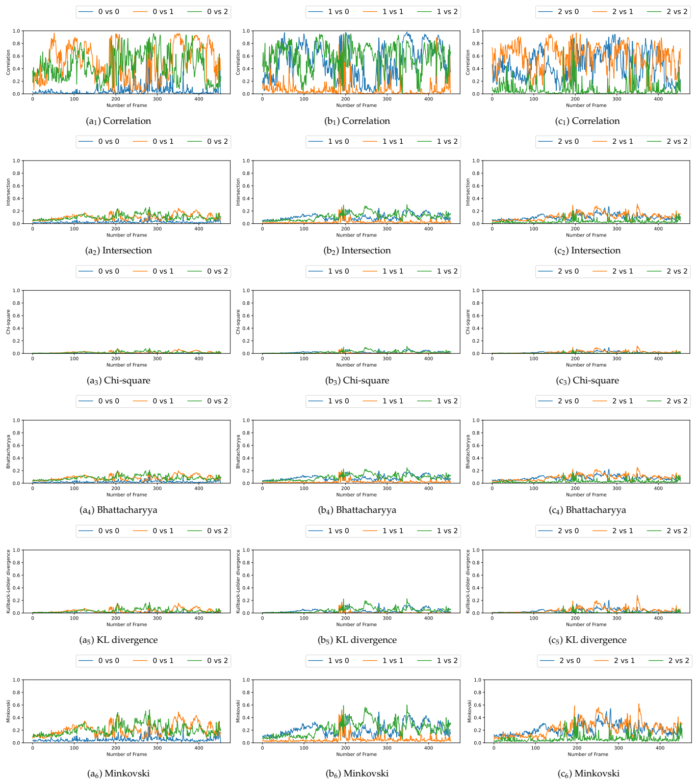
Figure 9. Curves comparing persons from one frame to another in video 2 (persons 0, 1, and 2) using the HOG.
