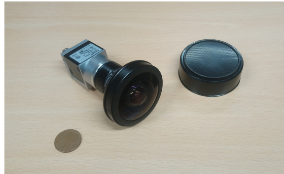
Figure 1. Basler ace acA2040-120uc color camera equipped with a fish eye lens utilized in our experiments. It is positioned next to a EUR 0.05 coin.
