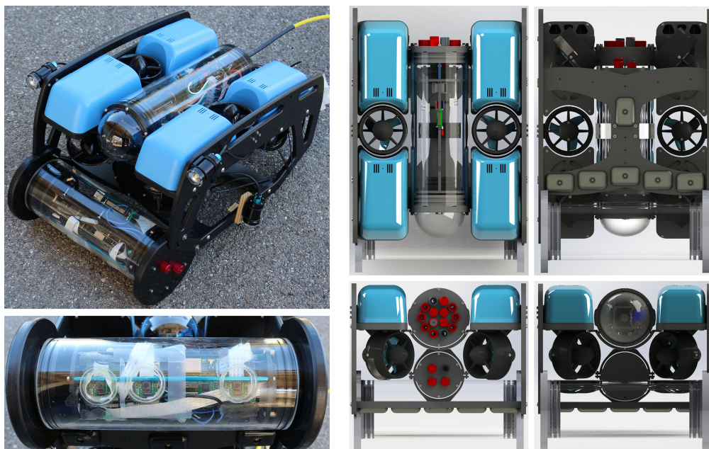
Figure 2. The built trifocal system integrated within a blueROV 2 (the front enclosure).
