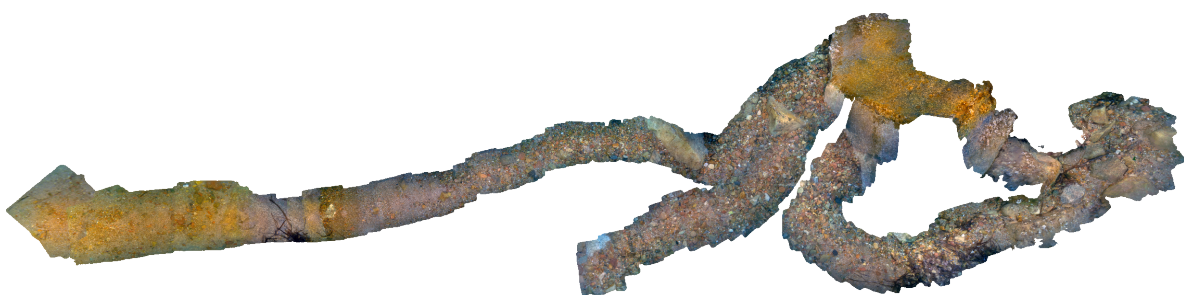
Figure 14. An example of the long trajectory 3D reconstructed model using images captured with the ROV-attached system. Such trajectories were used as ground truths to validate and tune the proposed method.
