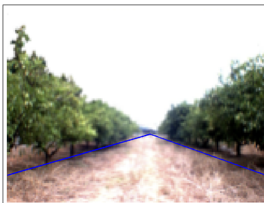
Figure 7. Detected border lines plot over the capture.
