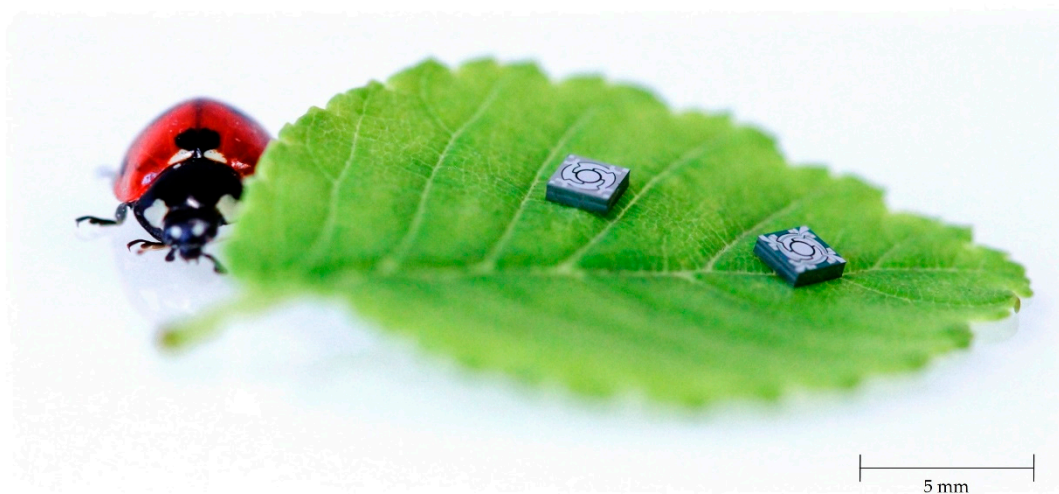
Figure 10. Diced micromirrors of Design 2 (left) and Design 1-S (right) in size comparison to a ladybug ( Coccinella septempunctata ).
