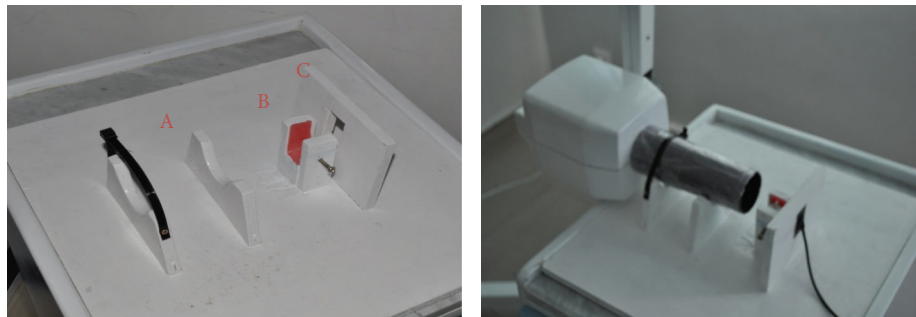
FIGURE 2: Fixation system. (A) Fixation zone of the radiological cone. (B) Fixation zone of the tooth. (C) Fixation zone of the radiological sensor.
