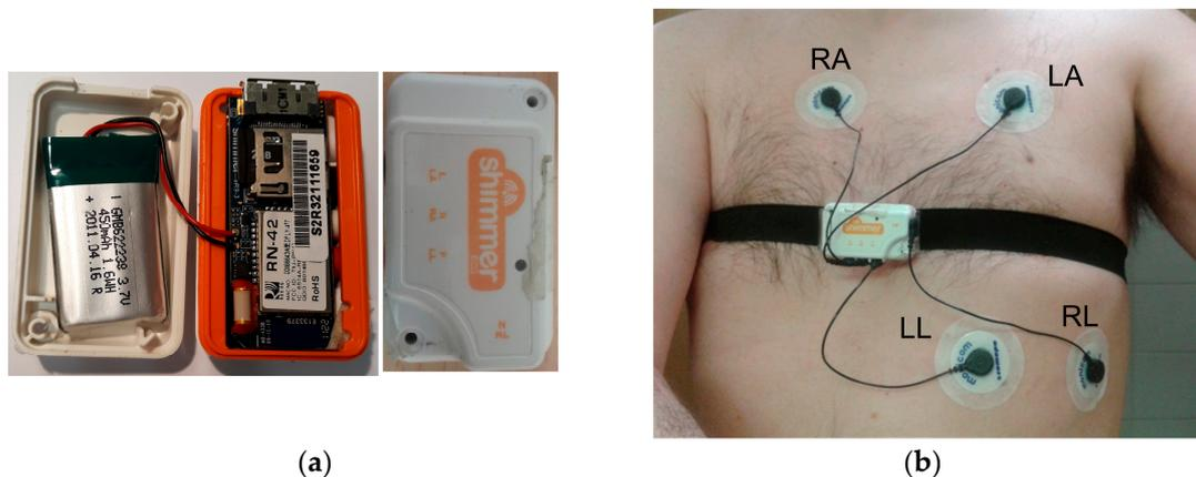
**Figure 1.** Shimmer electrocardiogram (ECG) sensor: (a) Shimmer ECG module; (b) Positions of the electrodes of the ECG sensor.
