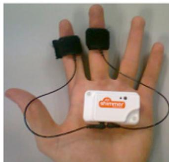
**Figure 3.** Position of the electrodes of the Shimmer galvanic skin response (GSR) sensor.
