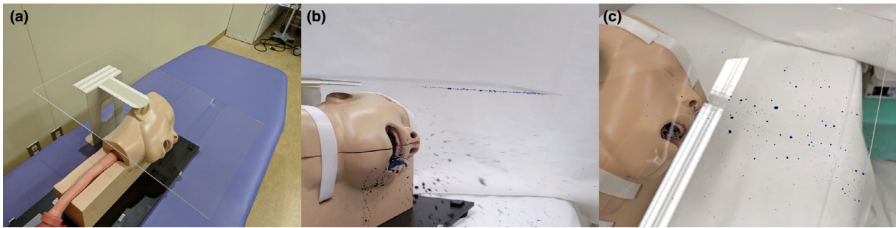
Figure 2 Image of a simulation to approximate a forceful cough generating droplets. (a) The device is placed to cover the patient's face and the space in front of the mouth. (b) Splashed droplets are blocked from spreading upward with the board. (c) The droplets adhere to the underside of the transparent board.
