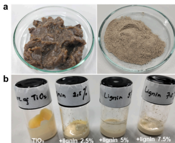
Fig. 1. Preparation of a) The water content removal of extracted rice husk result b) The composite of \text{TiO}_2 and lignin from rice husk.
